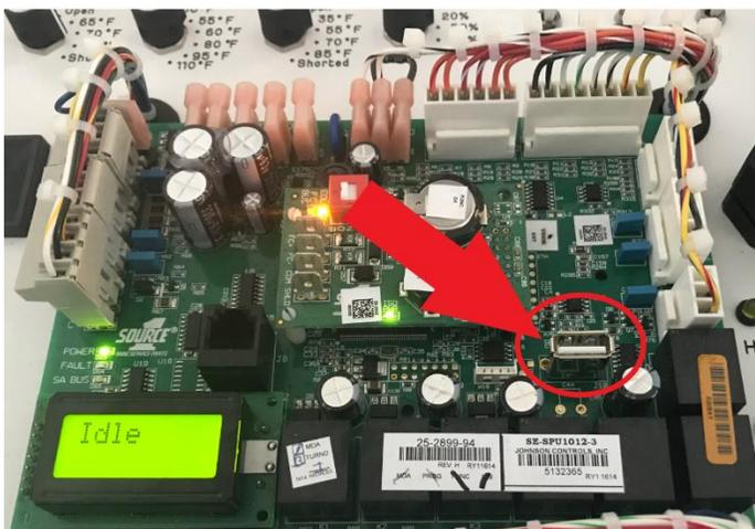
8. Through the local LCD display on the UCB with the joystick, navigate and select the firmware package to apply the update: Update>Load Firmware, select and confirm "4.4.1.3.secusb.pkg." Shown below in Figures 4 through 7.
